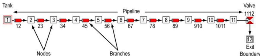
**Figure 4.** Finite volume GFSSP model of the flow network with single pipeline and valve
