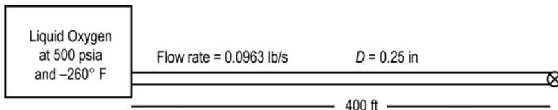
**Figure 3.** Schematic of the pipeline connected to a tank with an isolated valve placed at the end
